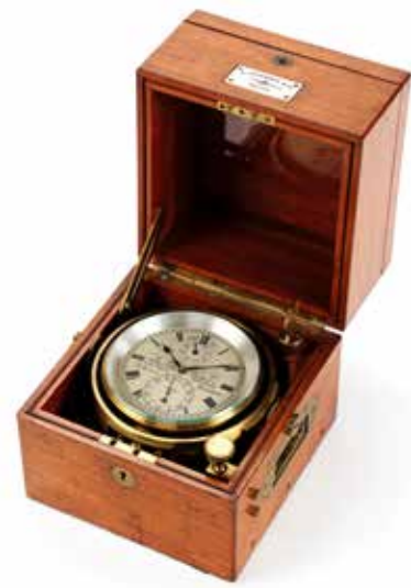
333 A GOOD EARLY 20TH CENTURY MAHOGANY CASED TWO DAY MARINE Y CHRONOMETER signed A. Johannsen & Co, no. 8109 the 3.5" silvered Roman dial with subsidiary dials for power reserve and running seconds, the movement with diamond endstone to the bimetallic balance with palladium helical hairspring and Earnshaw type detent escapement, with maintaining power to the chain fusee, 19cm high £1,000 - 2,000 €1,200 - 2,400
