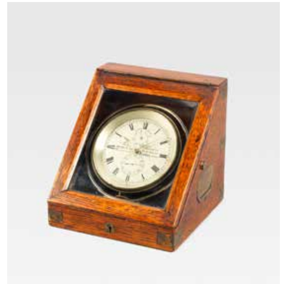
328 A 19TH CENTURY OAK CASED TWO DAY MARINE CHRONOMETER WITH FLETCHER'S PATENT AUXILIARY BALANCE signed John Fletcher, 148 Leadenhall Street, London, with 3.5" silvered Roman dial with state of wind and seconds dials, chain fusee movement, Earnshaw type detent escapement, 18cm high £1,000 - 2,000 €1,200 - 2,400
