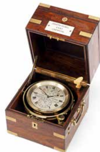
337 A GOOD LATE 19TH CENTURY ROSEWOOD TWO-DAY MARINE CHRONOMETER Y signed Joseph Sewill, 61 South Castle Street, Liverpool, No 4482 the 3.5 silvered Roman dial with minute track and twin subsidiaries for power reserve and running seconds, the chain fusee movement with freesprung diamond endstone, bimetallic balance and Earnshaw type spring detent escapement with maintaining power, 17cm wide £1,200 - 1,800 €1,400 - 2,100
