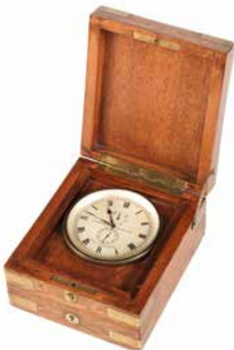
336 A 20TH CENTURY MAHOGANY CASED DECK WATCH WITH 36 HOUR POWER RESERVE signed Paul Ditisheim/ Chrono Solvil, the movement numbered 715617 the silvered 2.75" Roman dial with outer minute track and subsidiary dials for power reserve and running seconds, the frosted gilt bar 18-jewel movement adjusted to five positions with patented compensation and micrometer regulation, 12cm wide £800 - 1,800 €950 - 2,100
