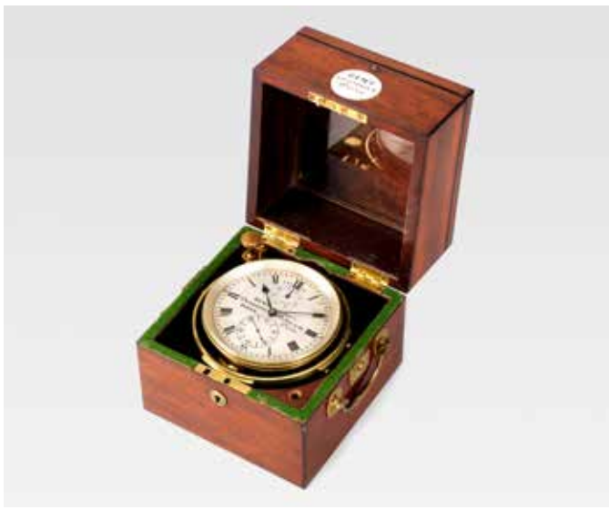
332 A MID 19TH CENTURY MAHOGANY CASED MARINE CHRONOMETER signed Dent, London, maker to the Queen No. 1779 the 4" silvered Roman dial with Roman numerals and subsidiaries for state of wind and seconds, the single chain fusee movement with Harrison's maintaining power and Earnshaw type detent escapement with Dents freesprung balance, 15.5cm wide £1,200 - 2,000 €1,400 - 2,400
